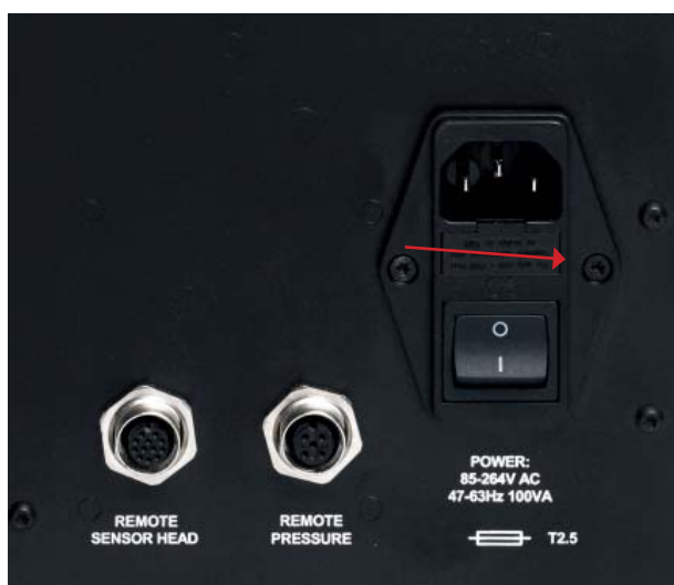
Figure 25 Power Supply Fuse Replacement
